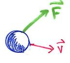
Instantaneous power delivered by a force:  $\mathcal{P} = F_{\parallel}v$ .
