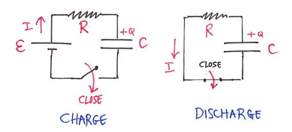
Charging capacitor in RC circuit:
